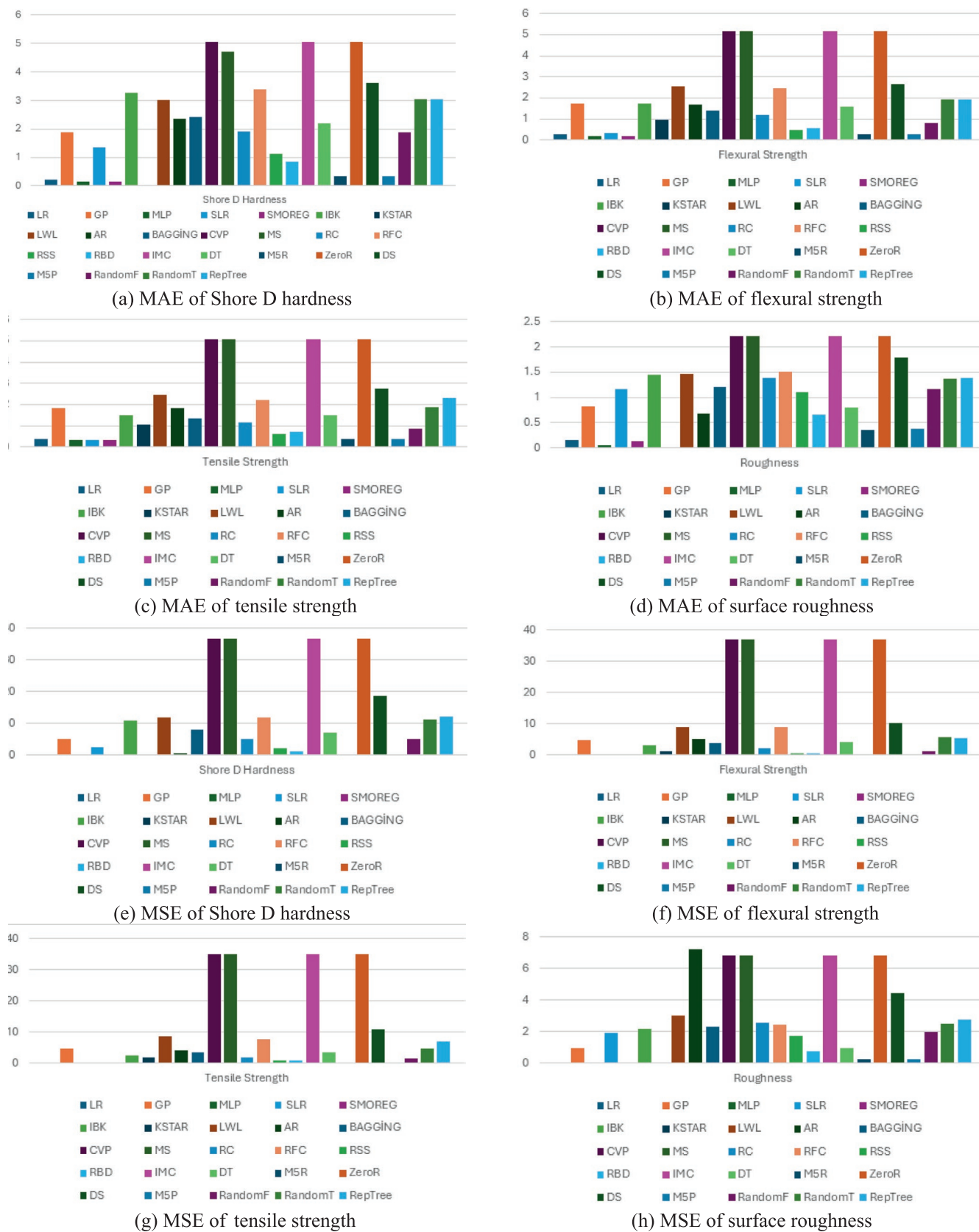
FIGURE 4 | MAE and MSE for predicting mechanical properties and surface roughness. [Color figure can be viewed at wileyonlinelibrary.com ]
