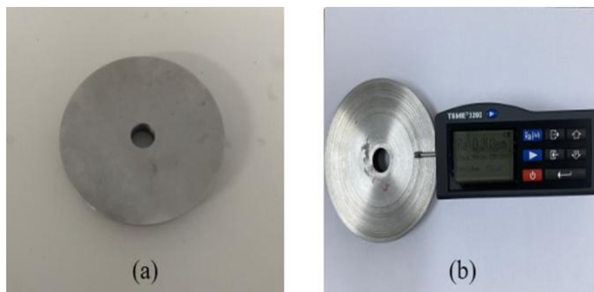
Figure 5. (a) Wear disk surface, (b) measurement of surface roughness of worn disk surface.
