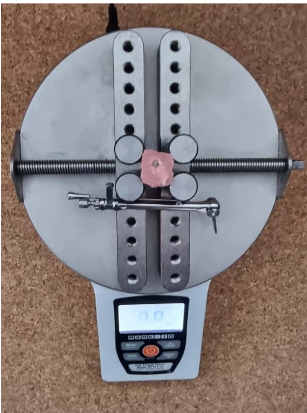
FIGURE 5. Measuring the osseointegration levels of implants with a reverse torque device (Mark 10, New York, USA).
