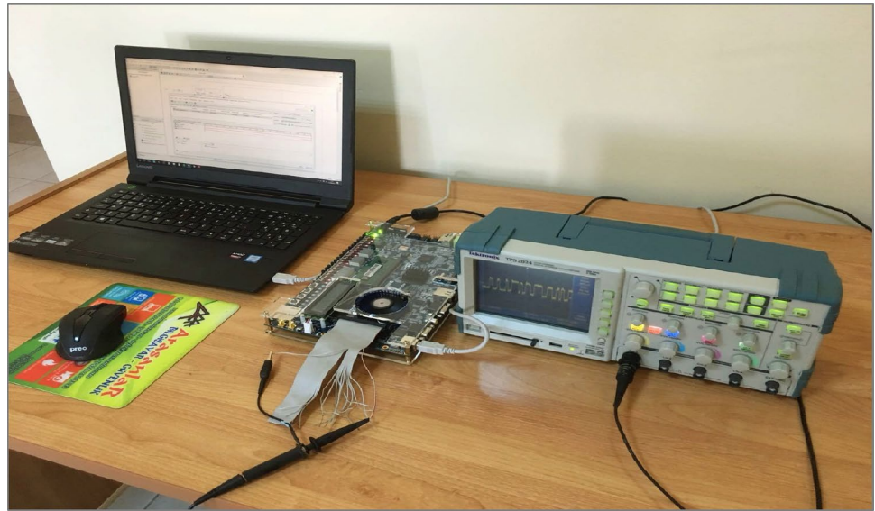
Fig. 4 Real-time experimental setup of the TRNG architecture
