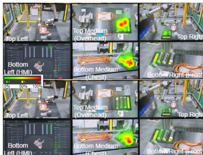
Figure 9. Operator gaze heat map during the experiments: top expert and bottom novice.
