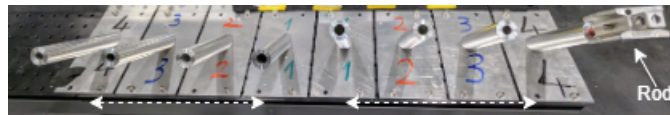
Figure 5. Multi-rod-in-tube task: the task difficulty varies based on the hole diameters (13.65 mm, 12.5 mm, 11.35 mm, and 10.2 mm) and the distance between the holes (100 mm, 300 mm, 500 mm, and 700 mm).
